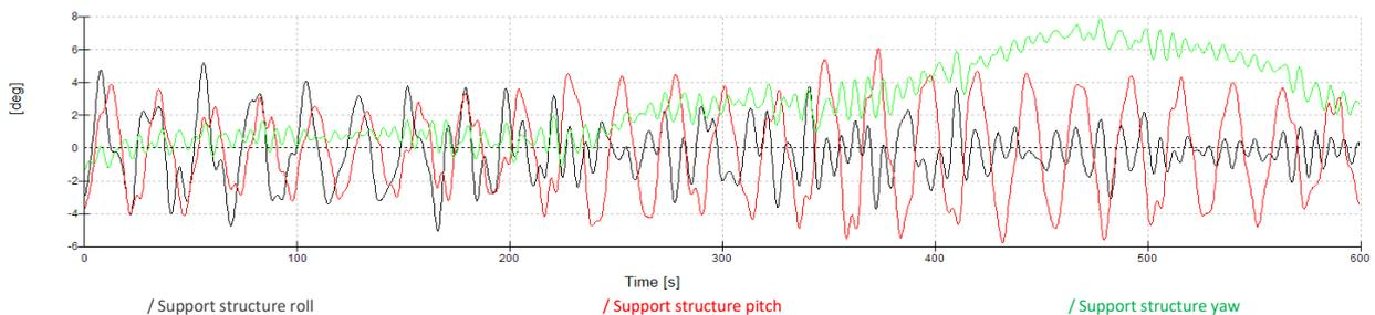
Figure 10 Displacements with waves and constant wind (case 2off<sub>a</sub>)
