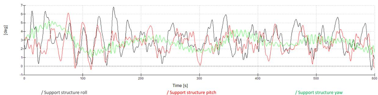
**Figure 12 Nacelle pitch, roll and yaw in normal operation vs. onshore @20-24 m/s**
